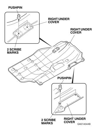
10. While wearing eye protection, drill the four piercings in the right under cover with a 3 mm drill bit.
