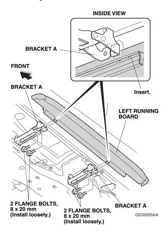
19. Tighten the four 8 x 20 mm flange bolts loosely secured in step 15. Torque the flange bolts to 22 N·m (2.2 kgf·m, 16 lbf·ft).
