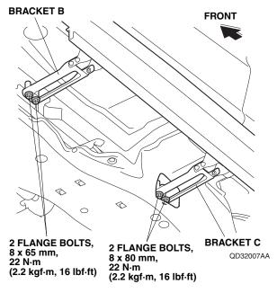
21. Tighten the four 8 x 20 mm flange bolts loosely secured in step 18. Torque the flange bolts to 22 N·m (2.2 kgf·m, 16 lbf·ft).
