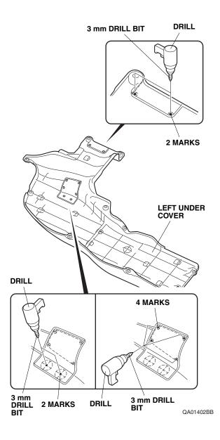
6. Enlarge six holes made in the left under cover in step 5 with a 6 mm drill bit, with an 8 mm drill bit, and finish with a 10 mm drill bit.
