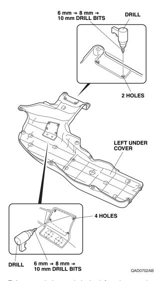
7. Enlarge two holes made in the left under cover in step 5 with a 30 mm hole saw. Remove any burrs.
