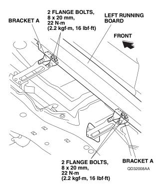
22. Tighten the eight 8 x 20 mm flange bolts loosely installed in step 17. Torque the flange bolts to 22 N·m (2.2 kgf·m, 16 lbf·ft).
