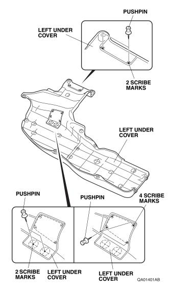
5. While wearing eye protection, drill the eight piercings in the left under cover with a 3 mm drill bit.
