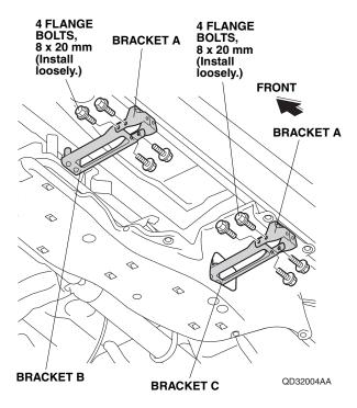
Secure the left running board to brackets A with four loosely installed 8 x 20 mm flange bolts.
